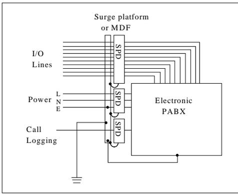
A much better solution is the creation of a surge platform where an exchange can take place without compromising the protection system. Consider the diagram on the left. Using this method, all bonding wires are kept very short and surge currents are exchanged on the surge
