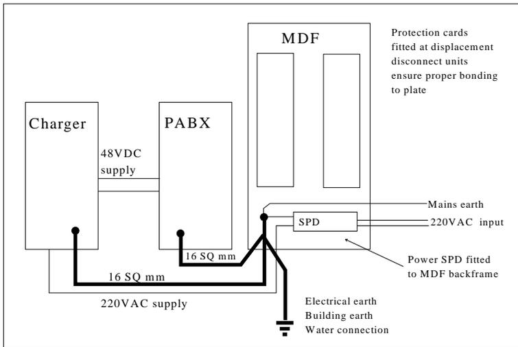
The distribution frame is used as the surge potential platform where the interchange of currents takes place. Even if the PABX unit is some distance away, it will be unaffected by surge currents, providing that all the inputs and outputs to the PABX pass through the distribution frame.
